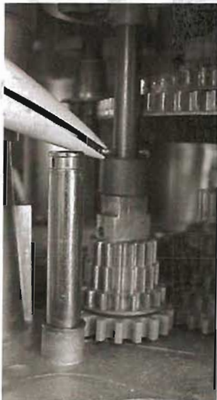
Lower spacer, re-install cotter pin
