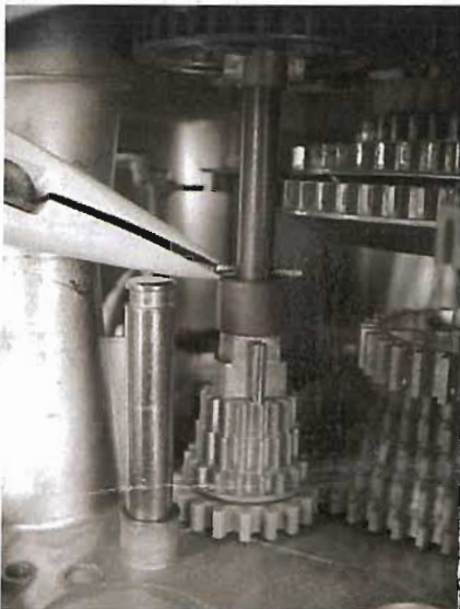
Remove cotter pin above spacer
