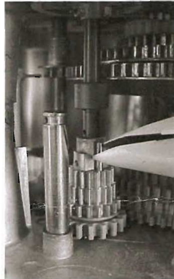
Lift spacer, remove Dollar Drive Shaft Vertical Pin
